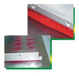
JB511-24 is one component epoxy resin with halogen free. It is one of special glue especially designed for surface mount device. Particularly suited where very fast cure is required on high speed SMT lines. According to the demand of which social effects of pollution, it is designed for use in Pb-Free soldering which require high temperature.
